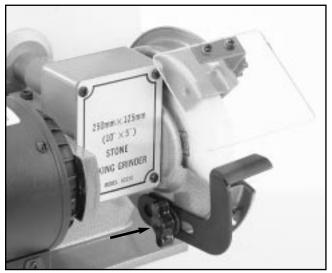
Figure 2. Knob to adjust tool rest.
